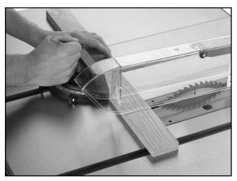
Figure 36. Cross-cut operation.
